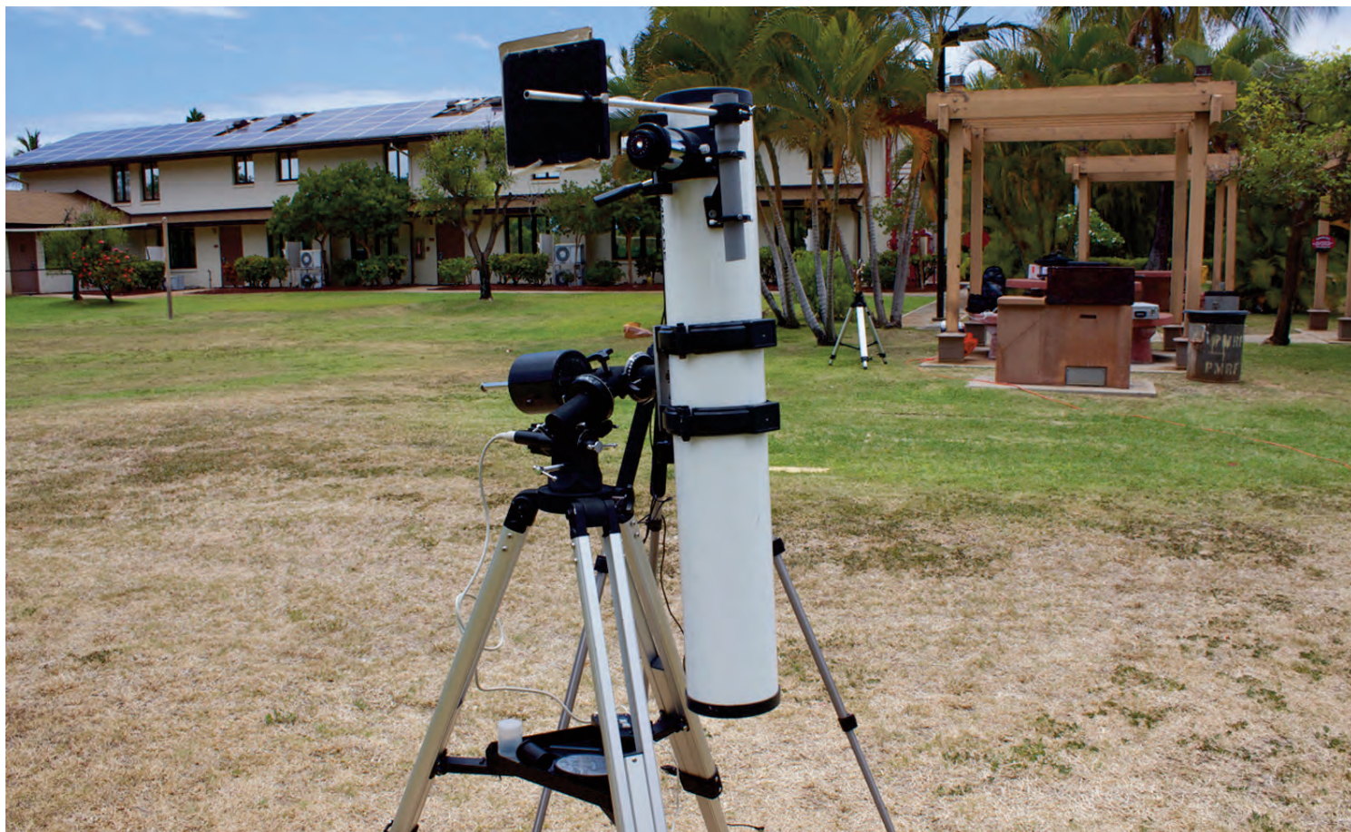
Image 11 Above - Here the author uses a six-inch Newtonian on a powered polar-aligned equatorial mount to project the Sun on a screen attached to the telescope.
